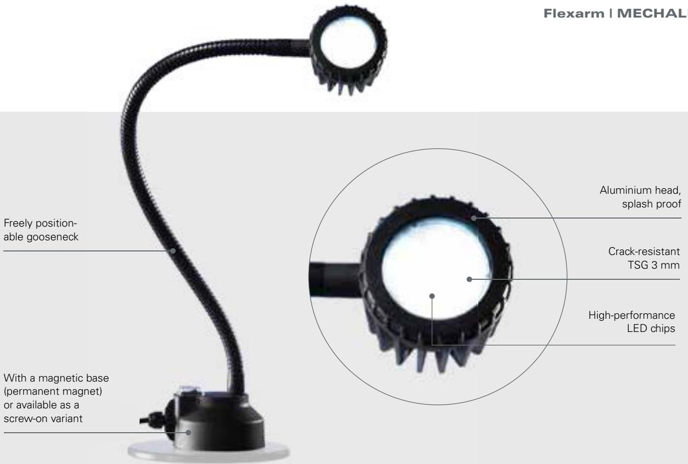
24V DC | III | 8.5 Watt | >750 lumens | IP64 | ≥80 | 5200K - 5700K | 60,000 h (L70/B10) | M12 | 3 m | +40 -10 | OPTION | 36 months | Germany
